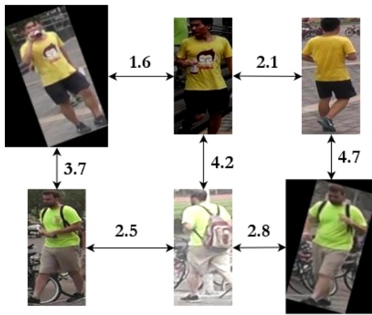
Fig. 10. Comparative study of feature distances in the presence of rotation and illumination variation. The intra-class feature distances is significantly lower compared to that of the inter-class feature distance. The feature distances are scaled by a value of 10^3
